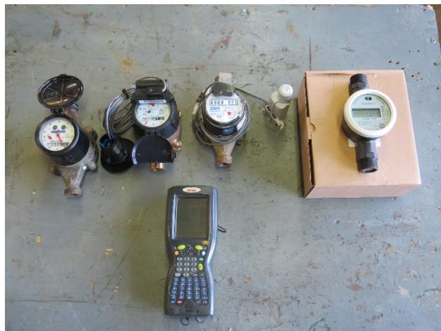
Figure 2. Typical Water Meters (top row l to r): direct read, touch pad, radio frequency, ultrasonic. Also shown below meters is an Itron MVRs hand-held data collection device.
